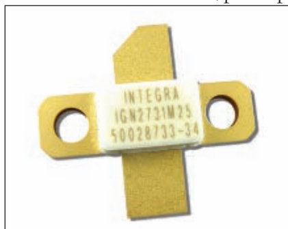
▲ Fig. 1 IG2731M25 produces over 25 W from 2.7 to 3.1 GHz (32 V, 300 \mu\text{s} and 10% duty cycle).
